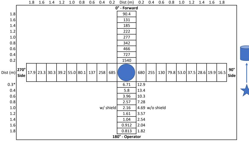
\*30 cm is the minimum object scatter-to-operator distance measurable
